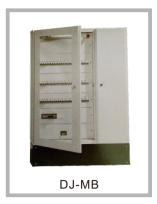
The 900mm width of frame with cable and busbar room, all parts are installed on the mounting plate. The busbar room can be chosen in the left or right side when installing the frame. Shield cover and door are constructed from 1mm galvanized steel with powder coated RAL7035.
