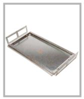
1.5mm galvanized mounting plate with many of 8mm dia holes, each two holes are 25mm distant. Galvanized steel are very good quality with excellent grounding performance.
